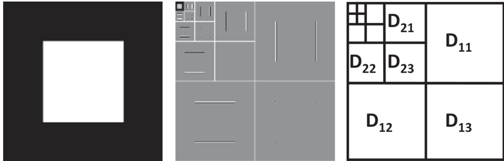
Fig. 6. Example on the directional sensitivity of the 2D Discrete Wavelet Transform (right: original image, center: DWT coefficients up to j=4 , left: correspondence between the DWT coefficients and the equations (11)-(14)).
